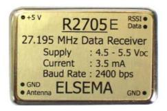
\*Only 66/33% duty cycle data is suitable for the R2705E receiver.
